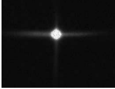
Figure 4.4: CO 2 -laser crossed dipole trap. Absorption image of the trapped atoms. The image is taken few microseconds after the end of the dipole trapping phase. More than one million of atoms are trapped with a temperature about 100 \mu K.
