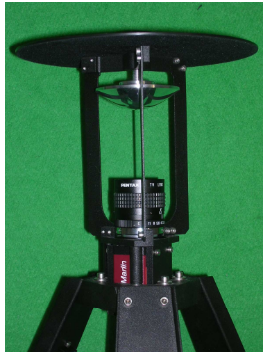
Figure 2.5: The omnidirectional vision system with a hyperbolic mirror and a Marlin F-046C camera.
