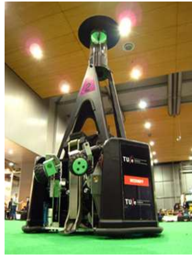
(b) Tech United Eindhoven robot 2008 . Two active wheels act as top dribblers, which can change the contact points on the ball and drive the ball in the longitudinal and lateral directions.
