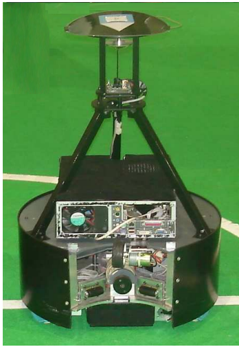
(a) CAMBADA robot 2007. One active wheel presses on the ball from above. Two inactive wheels are mounted on the front of the robot base.
