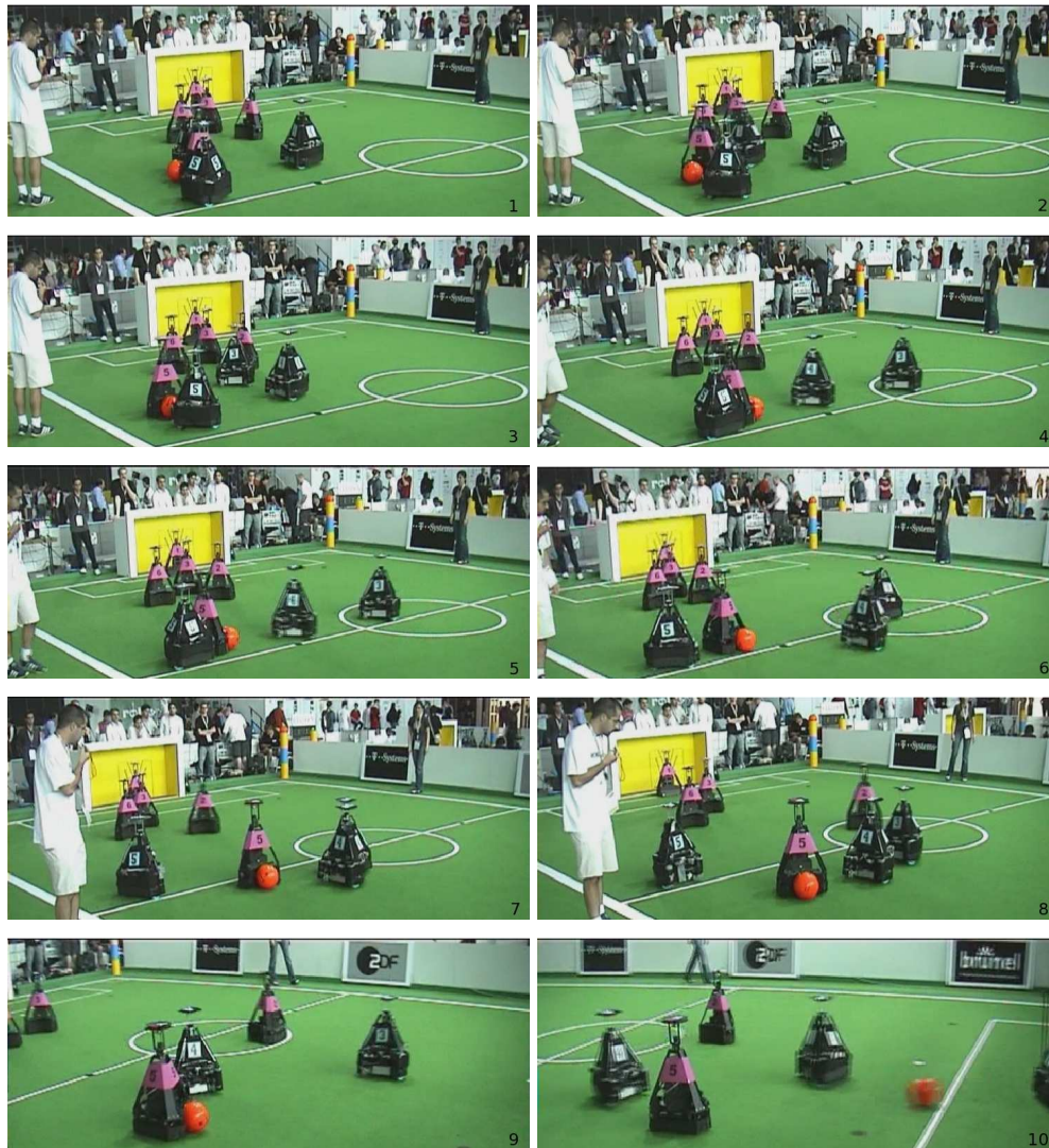
Figure A.10: Scenarios of a successful dribbling in the game against the AIS/BIT robots at the RoboCup World Cup 2006 in Bremen. The Attempto soccer robot No. 5 catches the ball in the neighborhood of two opponents, dribbles the ball out of this tight situation, avoids the third approaching opponent and finally shoots towards the goal. The images are sorted from left to right and from top to bottom.
