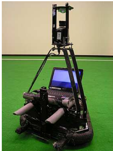
(c) Tribots robot 2006. The dribbling system consists of four rubber cylindrical bars representing the corners of an isosceles trapezoid.
