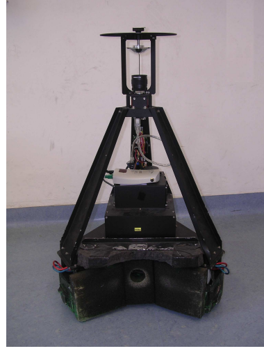
(f) Attempto robot 2006. A rubber foam pad is assembled above the concave robot front. Three spongy blocks are attached to the robot front to improve the damping property.
