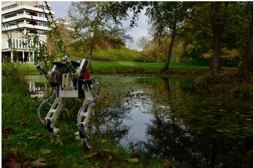
Figure 3.18: BirdBot can stand with its actuators switched off. Its foot latches and engages the leg mechanism, which in turn carries the robot's bodyweight. The foot provides a viable center of pressure, over which the center of mass can be positioned, see also Fig. 3.2C.
