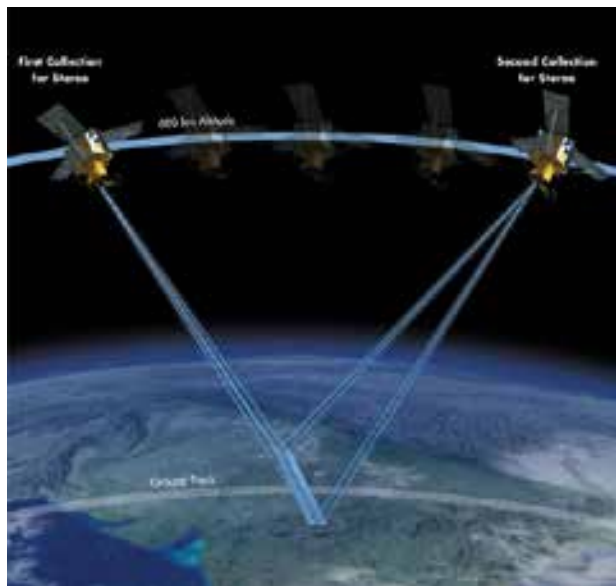
Figure 4. Acquisition method for capturing the topography with high-resolution stereo-image pairs of a linear array CCD sensor that takes images with one overfly. Same pass stereo pairs are advantageous for subsequent processing such as feature extraction because the scene content and lighting conditions are virtually the same for the two images. (Image courtesy Satellite Imaging Corporation).
