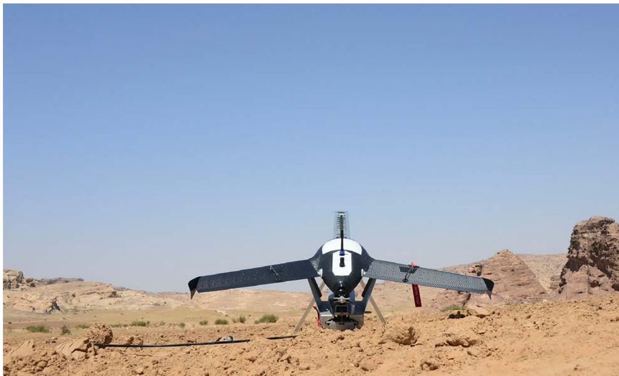
Figure 3. Photo of the Gatewing X100 fixed-wing UAS and catapult prior to take-off. The launch area was located approximately 2.5 kilometers northeast of the Ad Deir Plateau in the Al Beidha region. Photo courtesy of Bruce Allardice.
