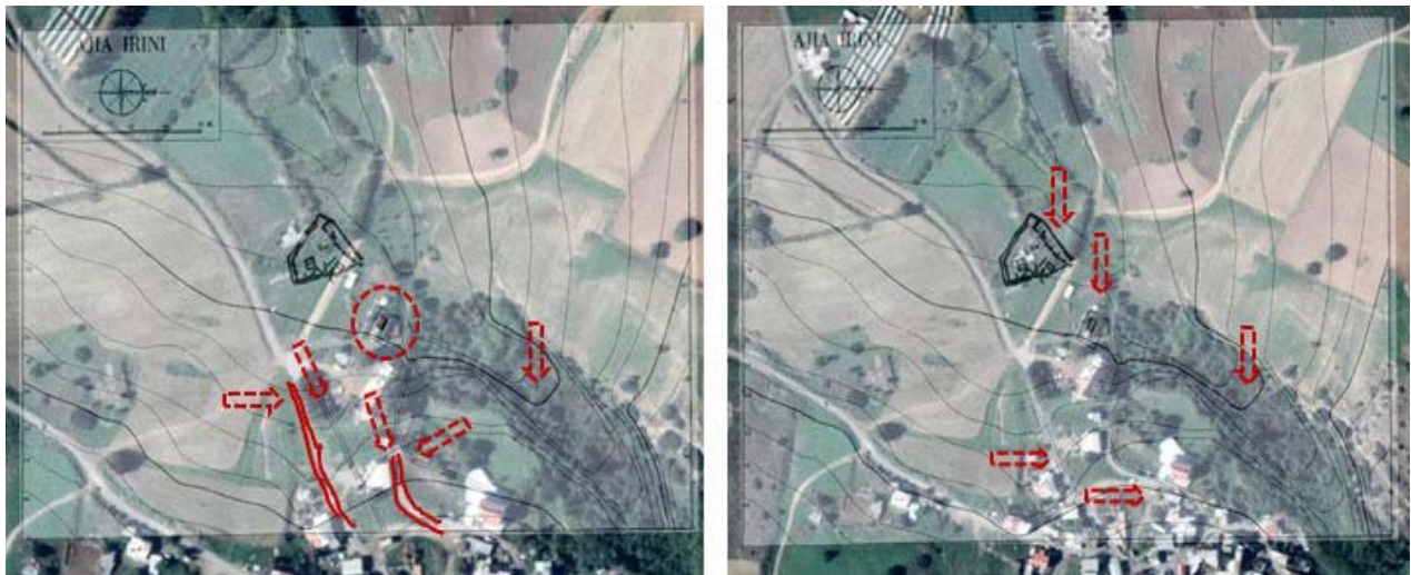
Figure 3. Georeference tests for finding the exact position of the sanctuary. The procedure brought to light the presence of measures' issues in the SCE plans (Vassallo©).
