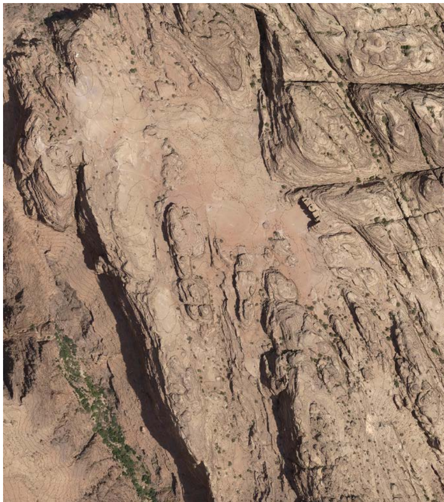
Figure 4. Orthomosaic generated by Pix4Dmapper from the images captured during the X100 flight. Contour lines were produced from a digital elevation model also created from the orthomosaic. The contour lines are shown superimposed over the orthomosaic.
