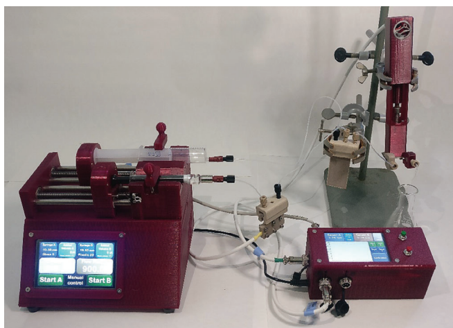
FIGURE 6 Flexible Open Source Microfluidic System (FOMSy), dual syringe pump, pressure sensor, automated pressure regulator, control unit, and PEEK microreactor. 10,11
