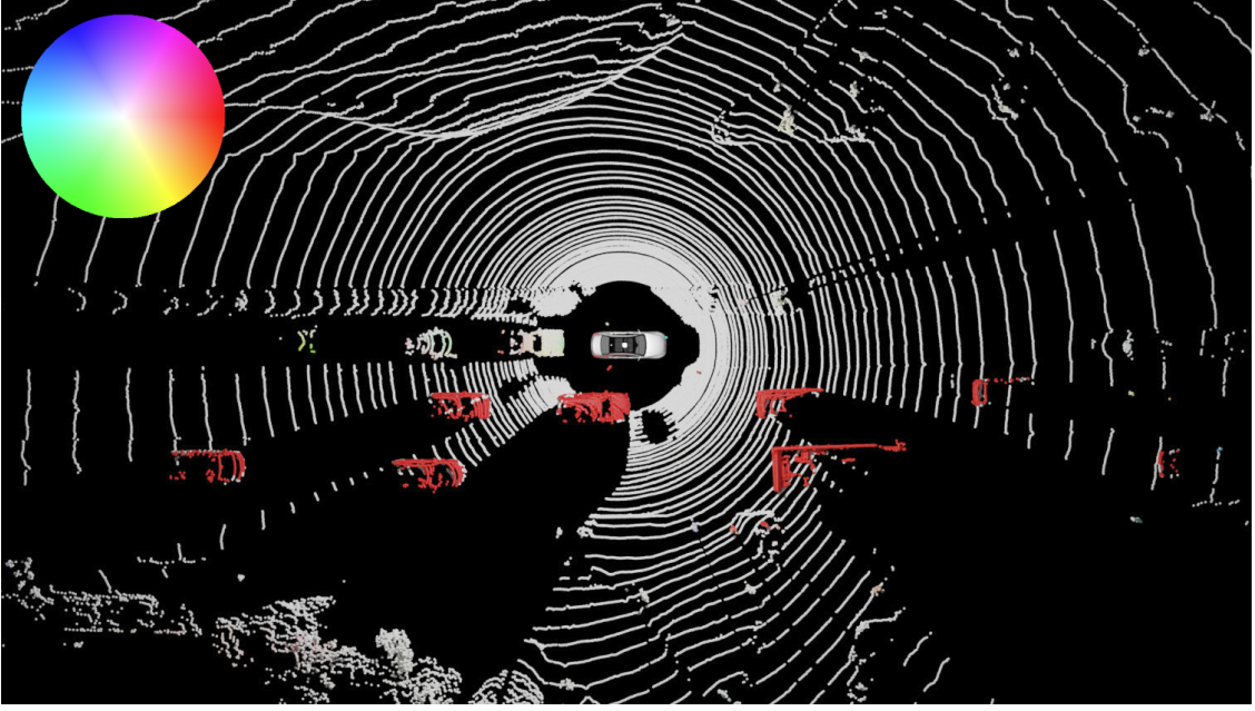
Figure 2.5: A point cloud with its corresponding LiDAR scene flow from the KITTI dataset. Ego vehicle is standing still, and the LiDAR scene flow is dominated by the forward motion of the cars (traffic is flowing towards the right in the image). The points are colored by the magnitude and orientation of the scene flow vector given the color wheel in the upper left corner.
