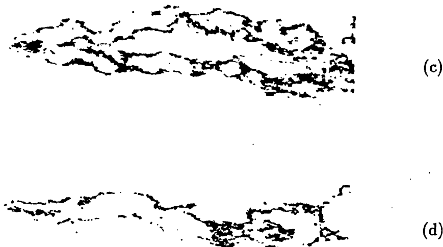
Fig. 2 Top view images of the bifurcated jets; (a) U_a=4.27 \text{ cm s}^{-1} , (b) U_a=5.64 \text{ cm s}^{-1} , (c) U_a=7.20 \text{ cm s}^{-1} , (d) U_a=11.36 \text{ cm s}^{-1} .
