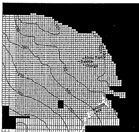
Fig. 2a Starting hydraulic heads, digitization of Ball's map 1927.
