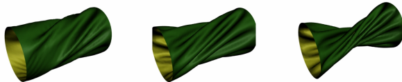
Figure 9: Torsional deformation of a cylinder. Notice the forming of folds starting with fine wrinkles which merge into bigger folds.
