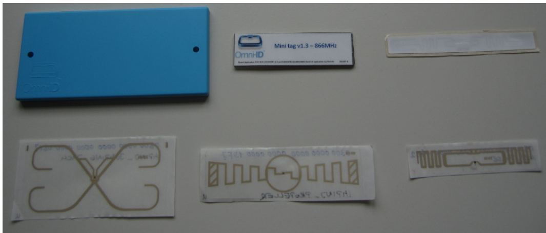
Figure 2.3: Examples of passive UHF RFID tags. Top (from left to right): OMNI-ID large tag, OMNI-ID small tag, and Alien Technology Squiggle tag. Bottom (from left to right): Impinj Jumping Jack tag, Impinj propeller tag, and NXP pulse tag.
