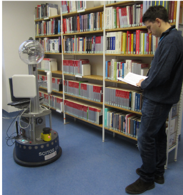
Figure 6.1: A scenario where our Scitos G5 robot is tracking a human carrying an RFID tag in a library.
