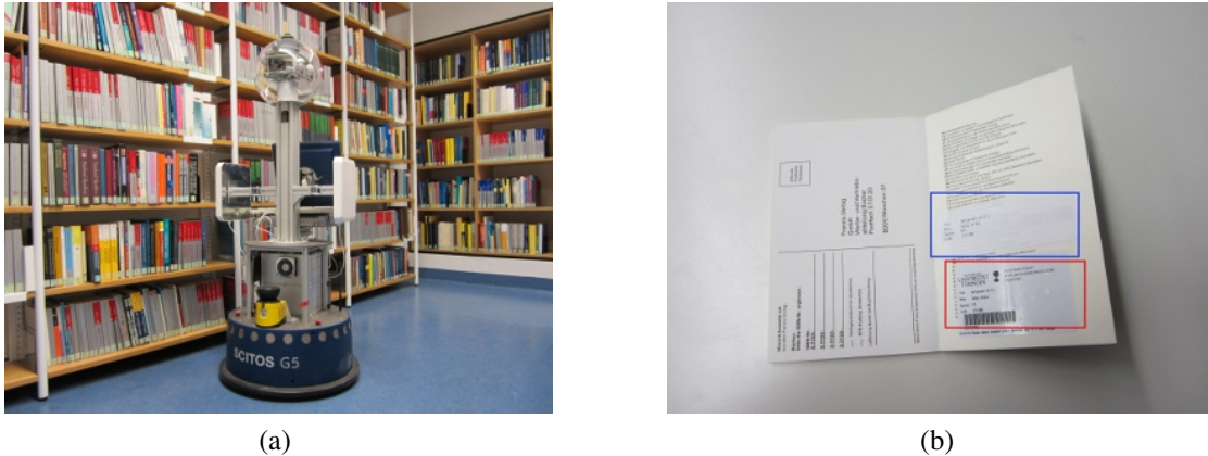
Figure 5.1: (a) RFID-tagged library scenario; (b) High frequency (HF, red) and ultra high frequency (UHF, blue) tags attached to the books. Only the passive UHF tags are used throughout our experiments - more information on the environment as well as the project (AmbiSense) can be obtained from http://www.ambisense.org .
