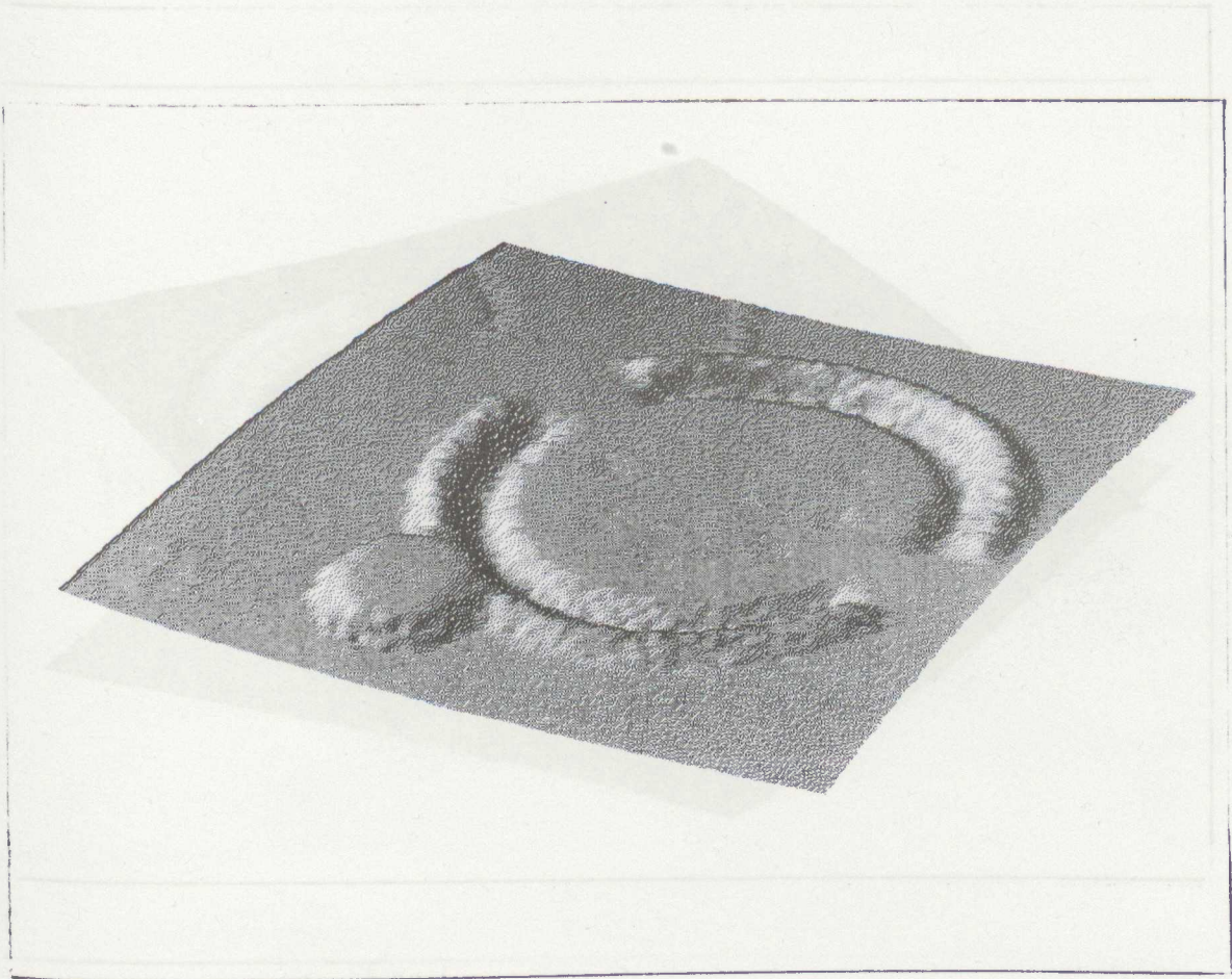
Figure 20.6: 100 \times 100 perturbed points, restored using fast interpolation.
